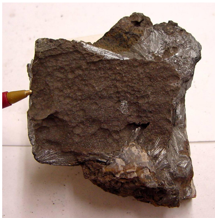
A pyrolusite specimen, composed principally of \text{MnO}_2 ; the pencil tip provides scale. Andrew Silver / USGS Mineral Specimens, via Wikimedia Commons, public domain.
