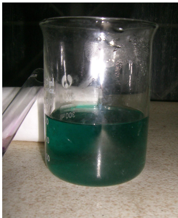
A deep-green manganate ( \text{MnO}_4^{2-} ) solution formed by treating hot potassium permanganate solution with sodium hydroxide. Choi / Wikimedia Commons, public domain.
