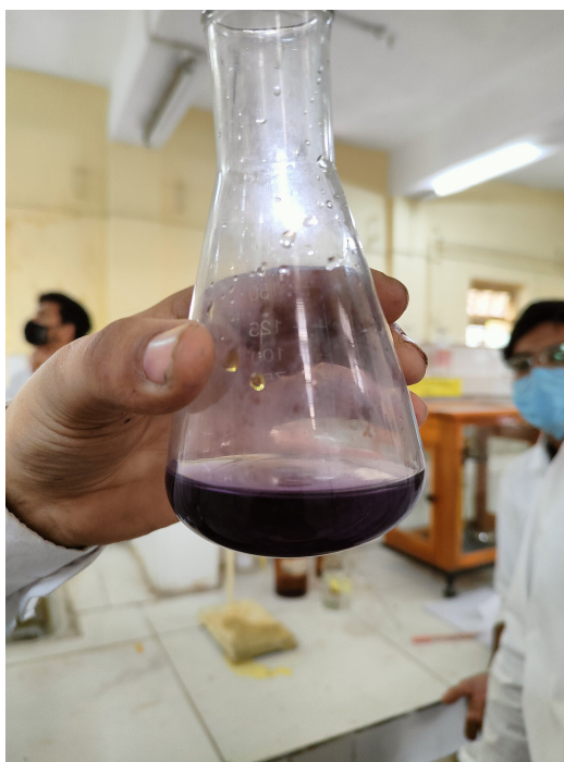
A potassium permanganate titration; the purple color is due to \text{MnO}_4^- . The original photograph does not identify the analyte, concentration, or stage of the titration, so the endpoint cannot be inferred from the image alone. Bhaiyaji Smile 123 / Wikimedia Commons, CC BY 4.0.
