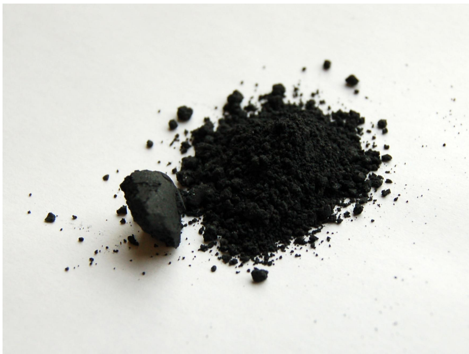
The characteristic black appearance of manganese dioxide ( \text{MnO}_2 ) powder. Benjah-bmm27 / Wikimedia Commons, public domain.
